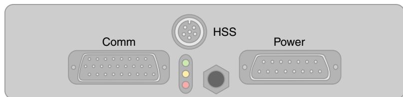
Figure 5-1: Diagram of the connectors on an ELCPU-PLUS or ELCPU layer including the 9-pin D-Sub Comm port used for serial bus inputs.
