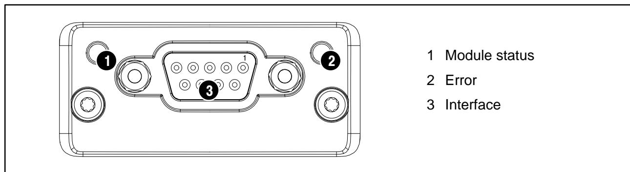
If both LED 1 and LED 2 are lit up red, a serious error has occurred and the interface has been deactivated (passive mode).
