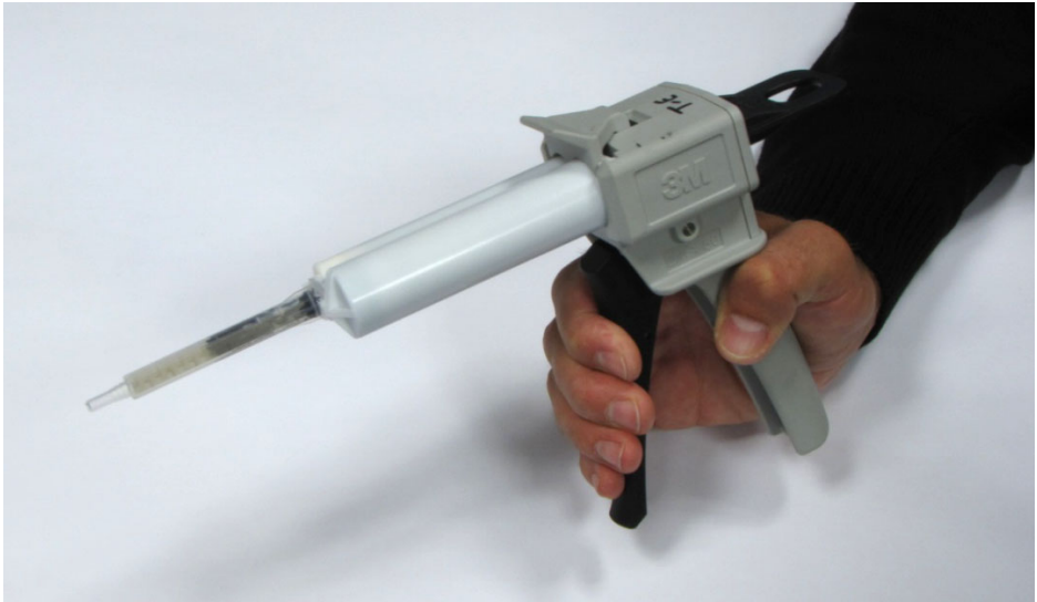
Fig. 3.4 Completed applicator with mixing nozzle attached
