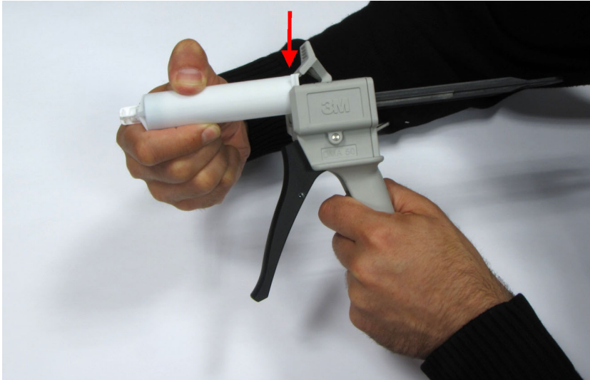
Fig. 3.2 Insert cartridge with adhesive
