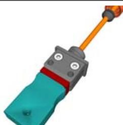
Push the arrangement into the ISOCAP (ensure correct polarity) and press in the grooved pins.
