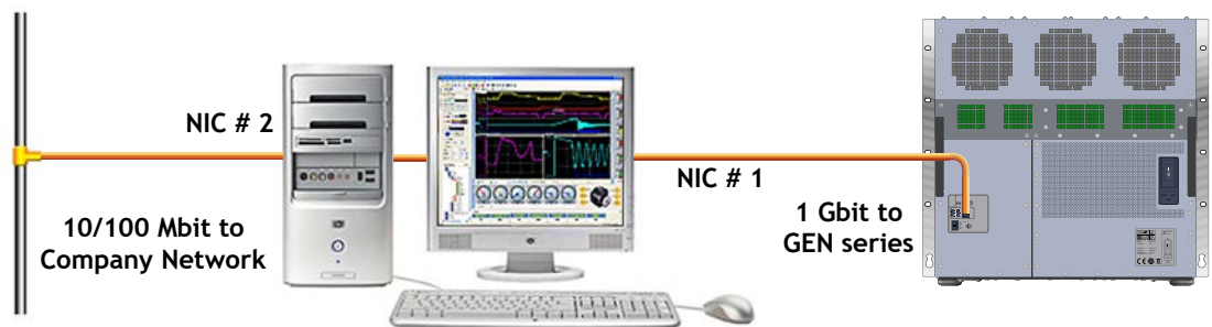
Figure 7.4: Direct connection to PC
