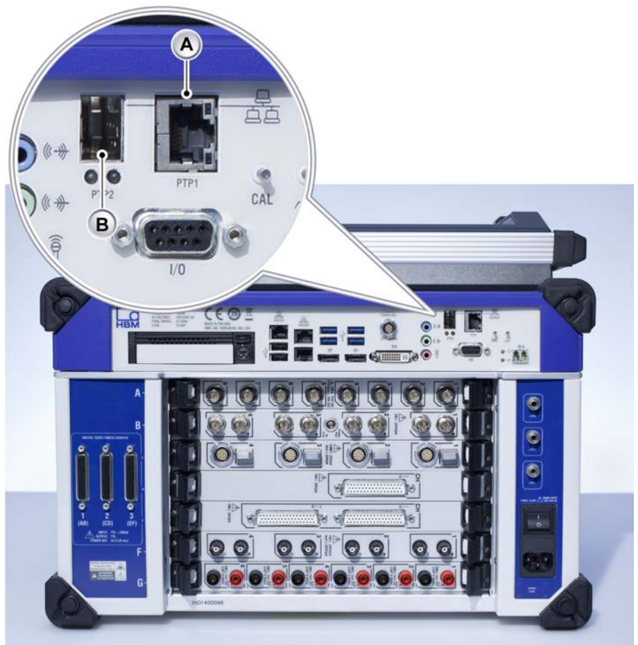
Figure F.1: GEN7i PTP enabled ports
