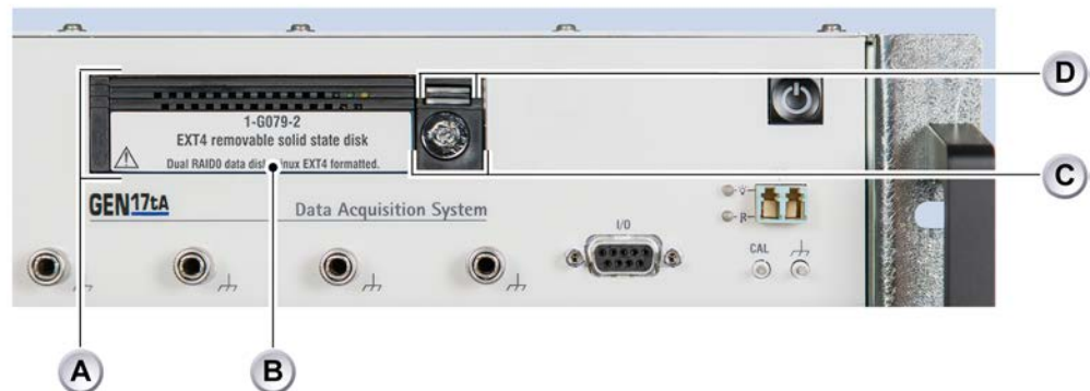
Figure 7.2: GEN17tA removable drive bay
