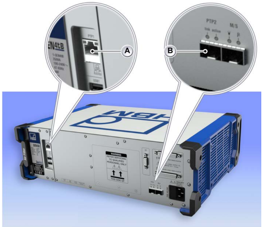
Figure F.5: GEN4tB PTP enabled ports
