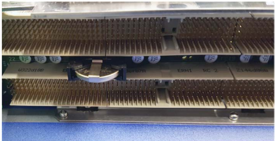
Figure 4.4: Battery in final position
