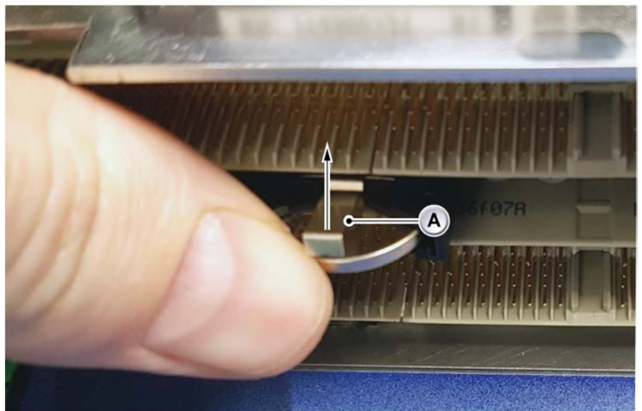
Figure 4.2: Lift Metal lid and pull out battery
