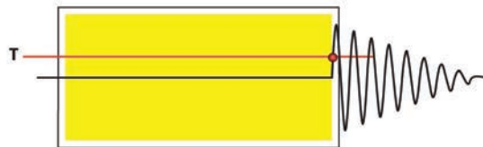
Figure 9.6: Full pre-trigger storage: pre-trigger = 100%
