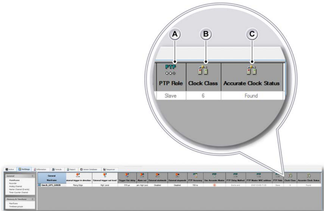
Figure 14.18: PTP synchronization status
