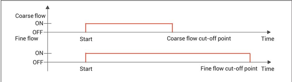
Fig. 11.3 Filling cycle with coarse + fine valve control
