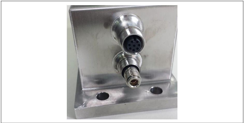
Fig. 5.1 Plug connection and (beneath it) the rapid-release coupling for connecting the air pressure equalization
