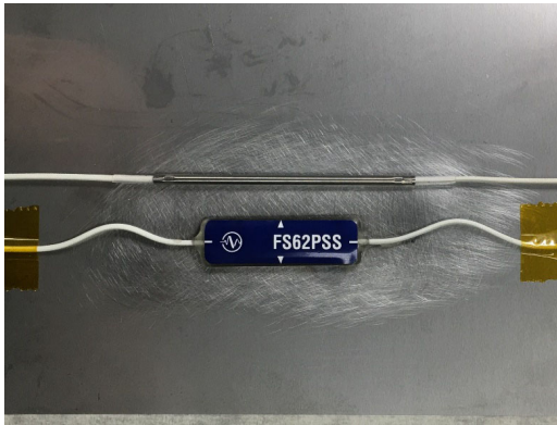
Fig. 2.22 Positioning the temperature sensor
