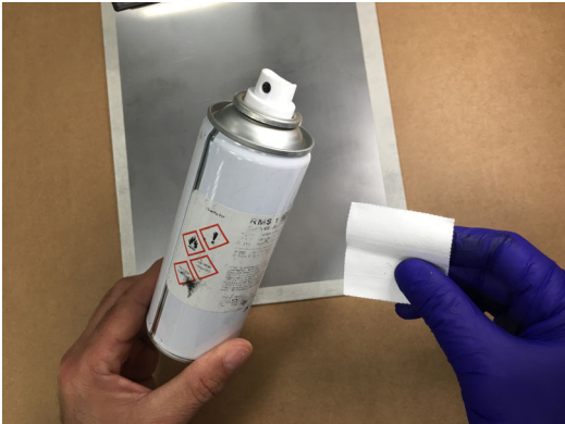
Fig. 2.3 Using RMS1 cleaner and nonwoven tissues
