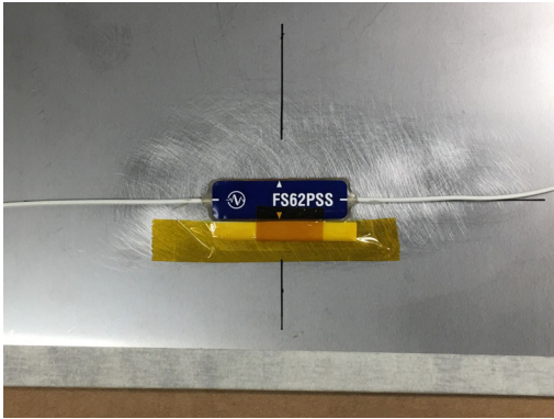
Fig. 2.8 Aligning and placing the FS62PSS
