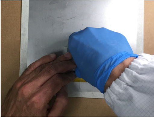
Fig. 2.20 Pressing on the rosette for 1 minute
