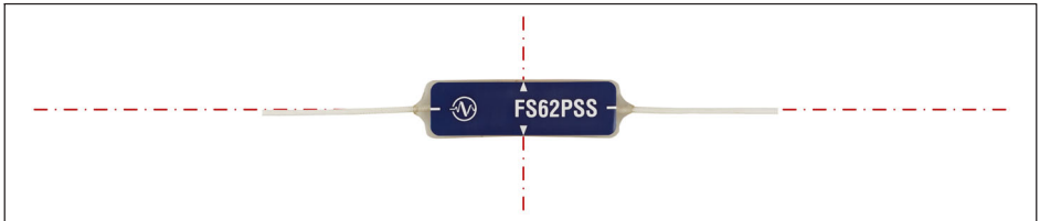
Fig. 2.6 FS62PSS Sensor alignment markings
