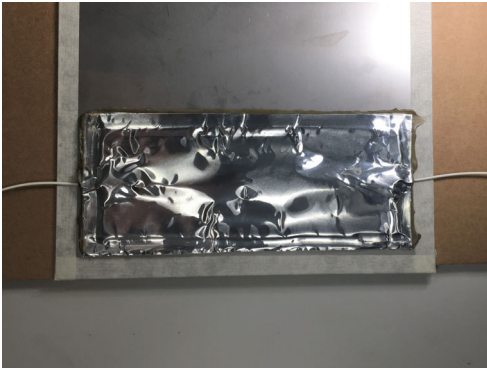
Fig. 2.31 Completely covered measuring point
