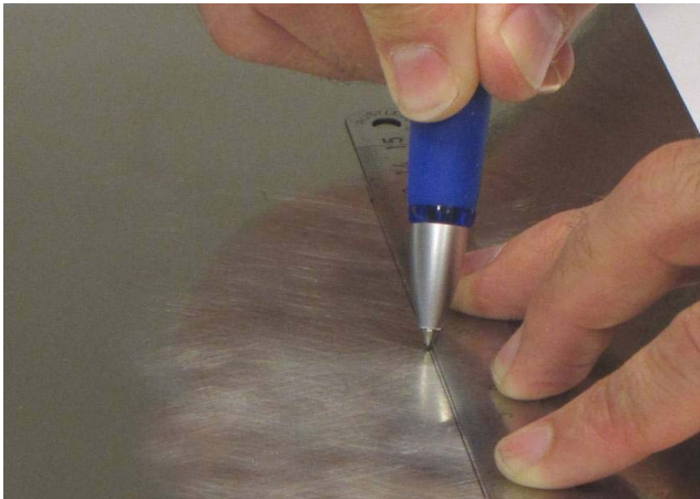
Fig. 2.8 Making the marking lines
