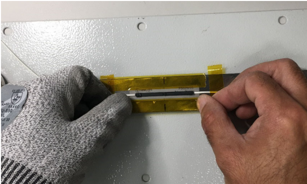
Fig. 2.11 Ensuring a smooth welding process by thoroughly fixing the sensor
