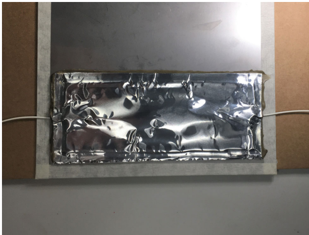
Fig. 2.31 Completely covered measuring point
