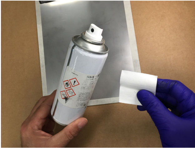
Fig. 2.5 Using RMS1 cleaner and nonwoven tissues
