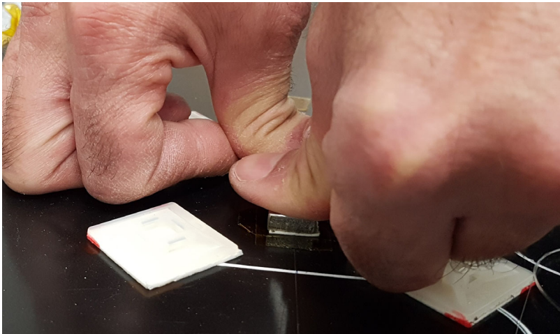
Fig. 2.19 Applying uniform pressure over the FBG.
