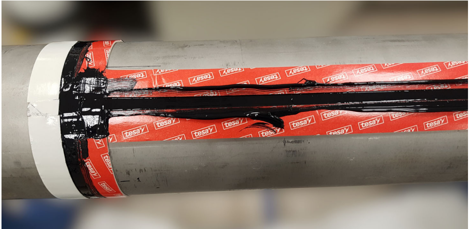
Fig. 2.21 Spreading the glue with a spatula.
