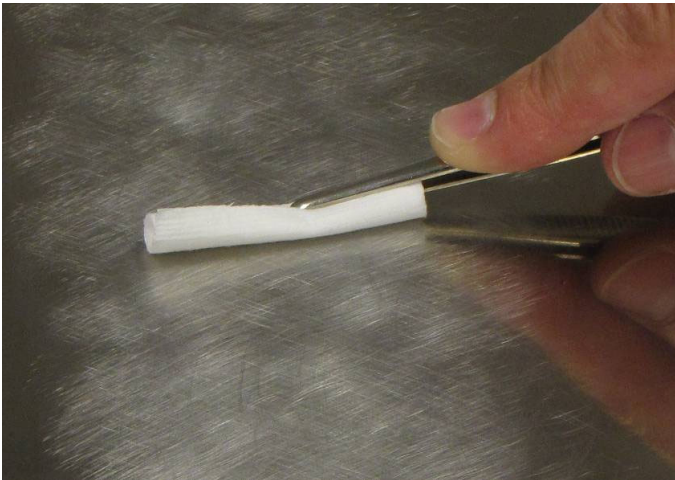
Fig. 2.4 Cleaning the roughened installation surface
