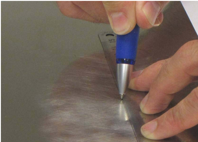
Fig. 2.6 Marking the marking lines
