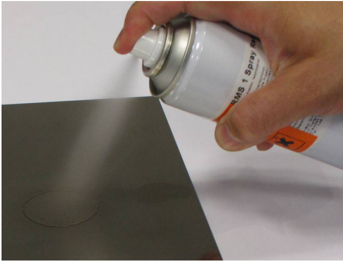
Fig. 2.1 Spraying 1-RMS on specimen
