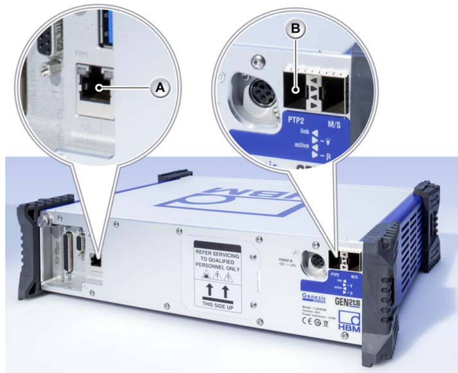
Figure F.4: GEN2tB PTP enabled ports
