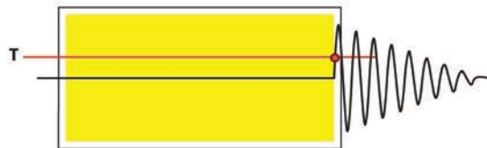
Figure 9.6: Full pre-trigger storage: pre-trigger = 100%
