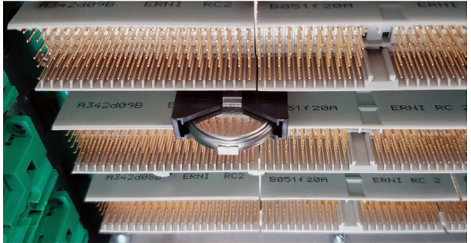
Figure 4.3: Battery in final position
