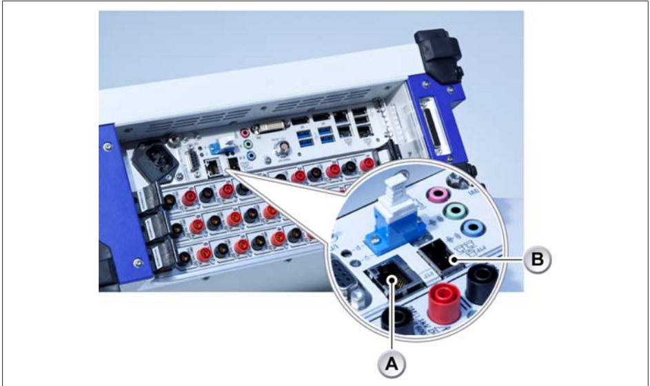
Fig. G.6 GEN3i PTP enabled ports
