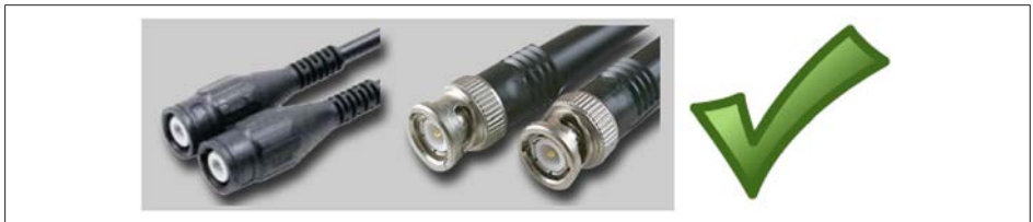
Fig. 13.56 Safe connectors for use with Isolated Basic acquisition cards
