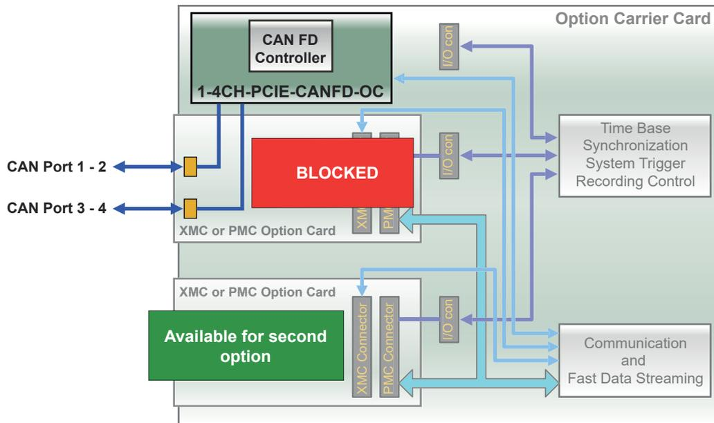
Figure 1.25: Block diagram 1-4C-PCIE-CAN FD-OC (G081 required)
