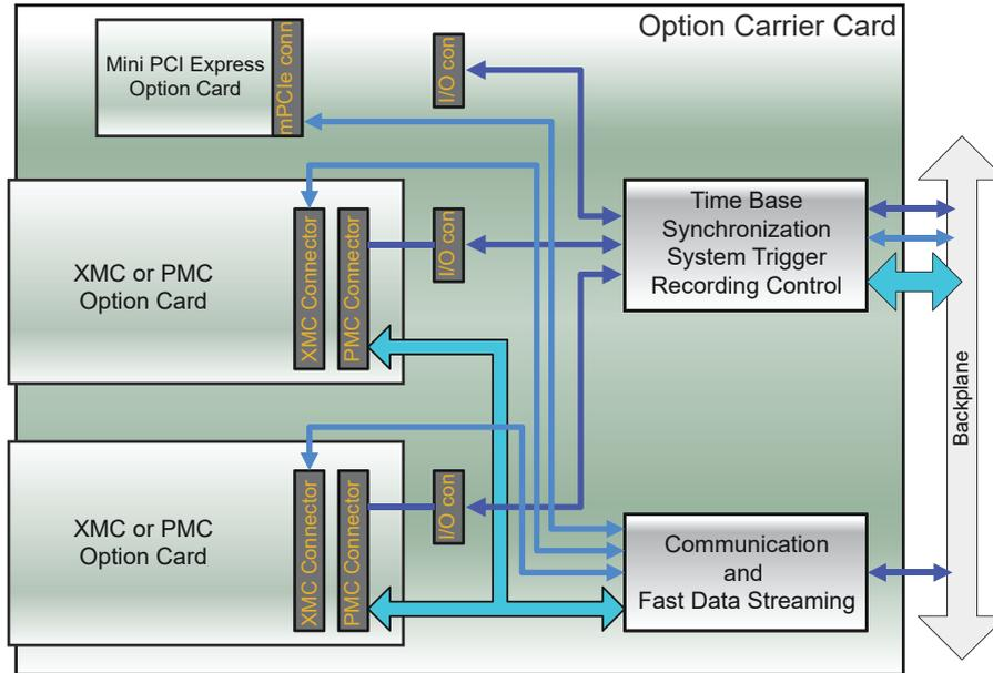
**Figure 1.21:** Block diagram option carrier card
