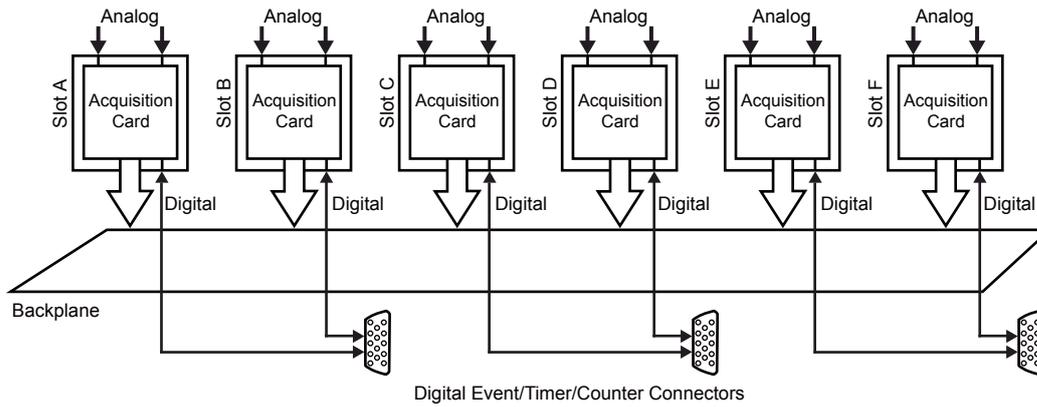
**Figure 1.13:** Digital Event/Timer/Counter block diagram
