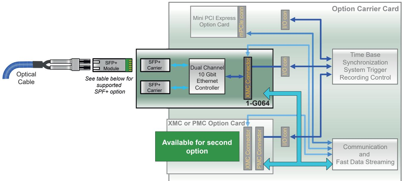
Figure 1.22: Block diagram 10Gbit Ethernet card, optical (G081 required)
