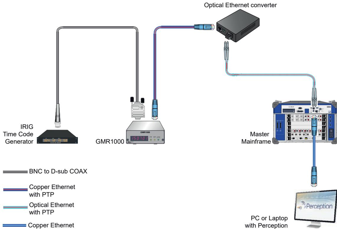
**Figure 1.34:** Example setup IRIG time synchronization
