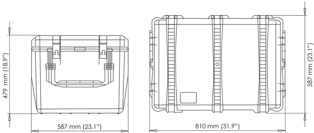
**Figure 1.38: Reusable hardcover shipping case with wheels and transport handle**
