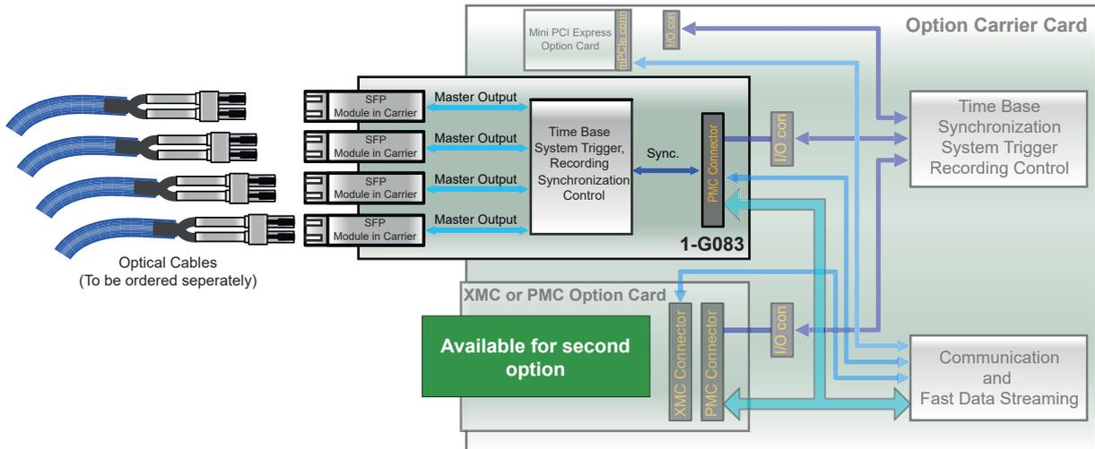
Figure 1.23: Block diagram Master output card (G081 required)
