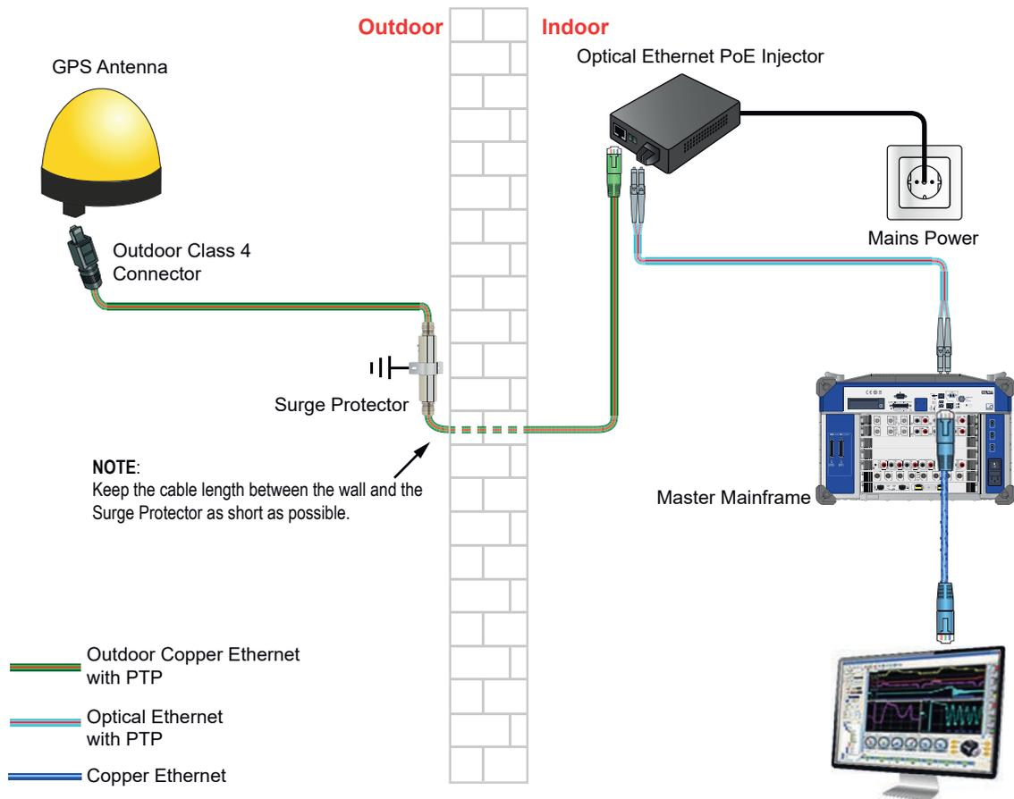
**Figure 1.35:** Example setup GPS time synchronization
