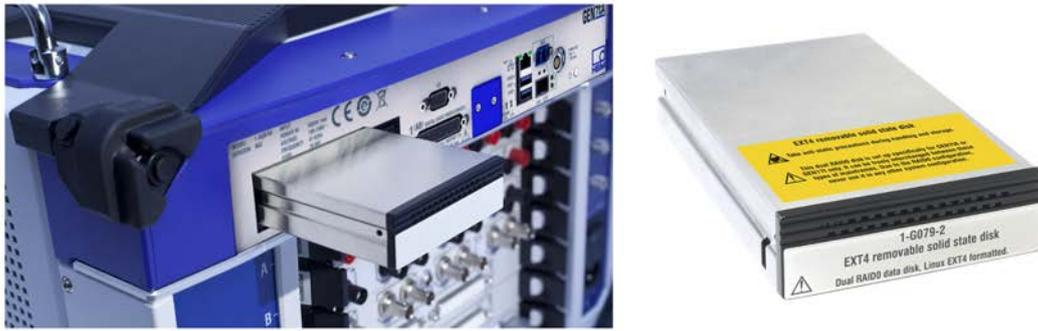
Figure 1.19: Example of SSD in drive carrier partially slid into GEN7tA (left) and SSD built inside drive carrier (right)
