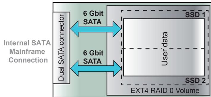
Figure 1.20: Block diagram drive
