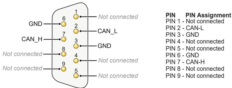
Figure 1.28: Pin assignment D-Sub
