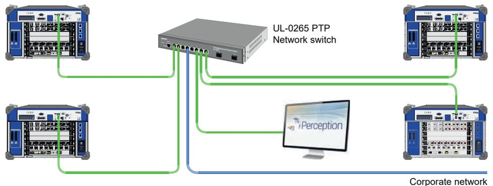
Figure 1.5: Multi mainframe (distributed)
