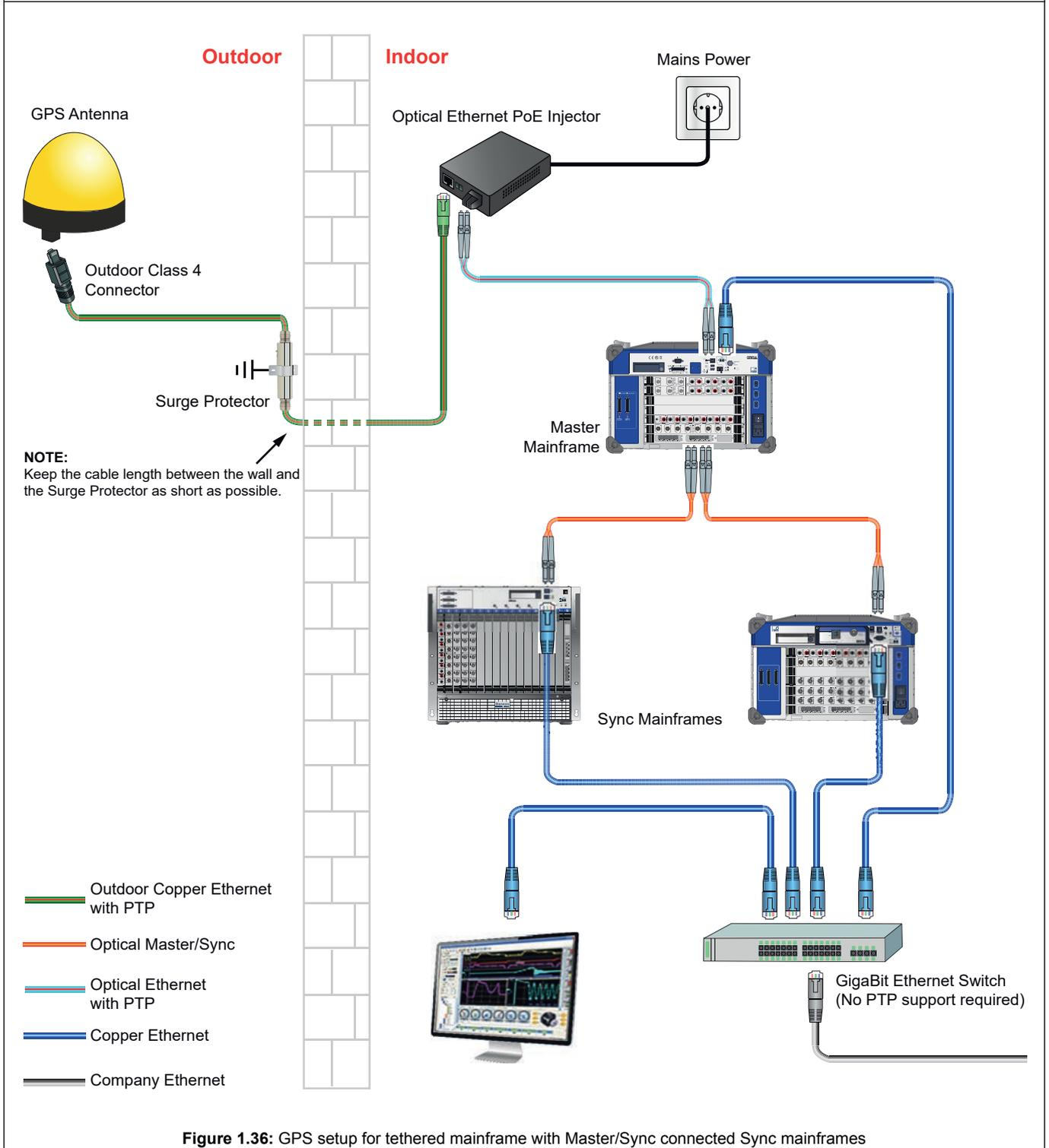
**Figure 1.36:** GPS setup for tethered mainframe with Master/Sync connected Sync mainframes
