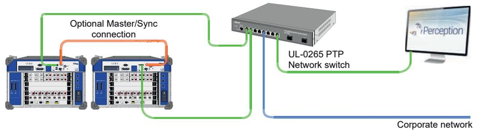
Figure 1.3: Dual mainframe
