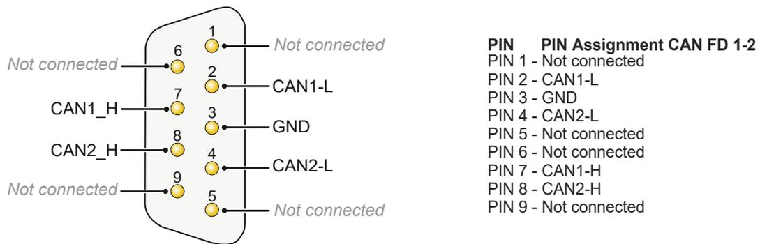
**Note:** For pin assignment for CAN FD 3-4 replace **CAN1** with **CAN3** and **CAN2** with **CAN4**
