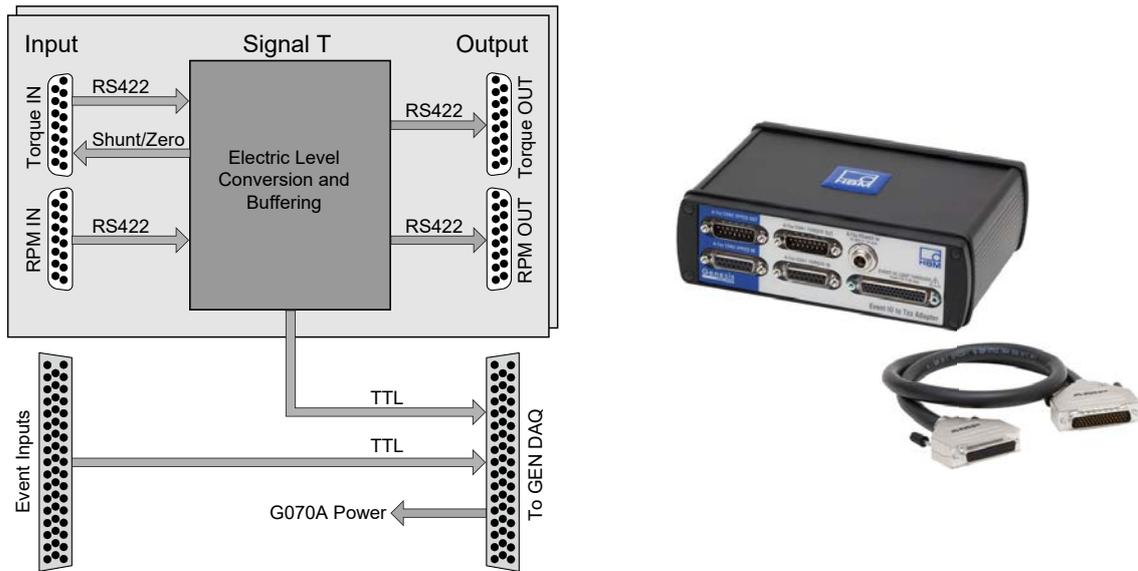
Figure 1.32: Block diagram and image
