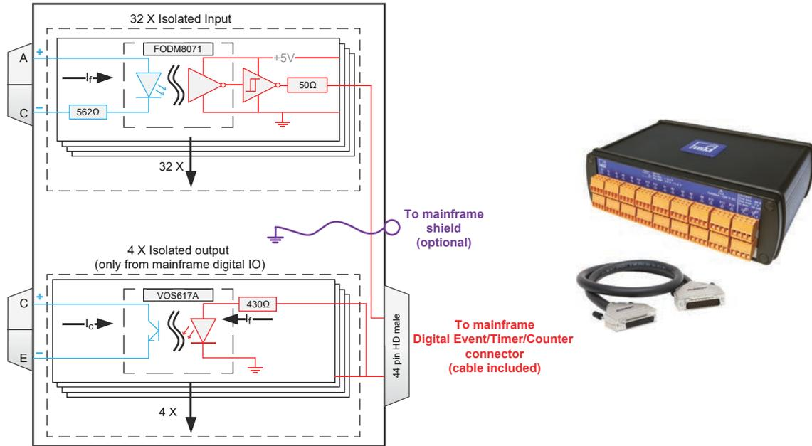
Figure 1.33: Block diagram and image
