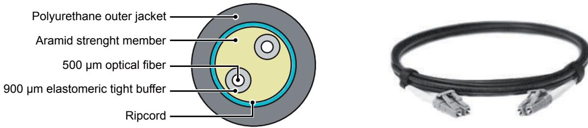
**Figure 1.31:** Block diagram and image
