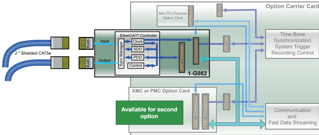
Figure 1.24: Block diagram EtherCAT® card
