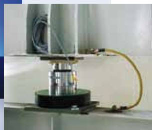
RTN load cell with elastomer bearing below a tank bracket
