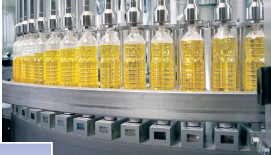
FIT® load cells enable bottling plants to be optimally controlled through the conditioning of measurement signals
