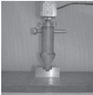
Fig. 5.1.1-2: Determining the interlaminar shear strength ILS
