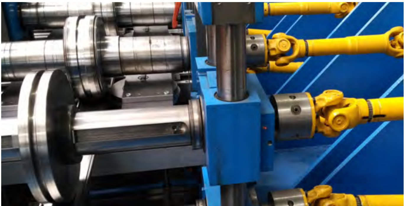
With an accurately selected measuring point (e.g. the yellow drive shafts), the surrounding parts (bearings, shafts and roller) can also be monitored.
