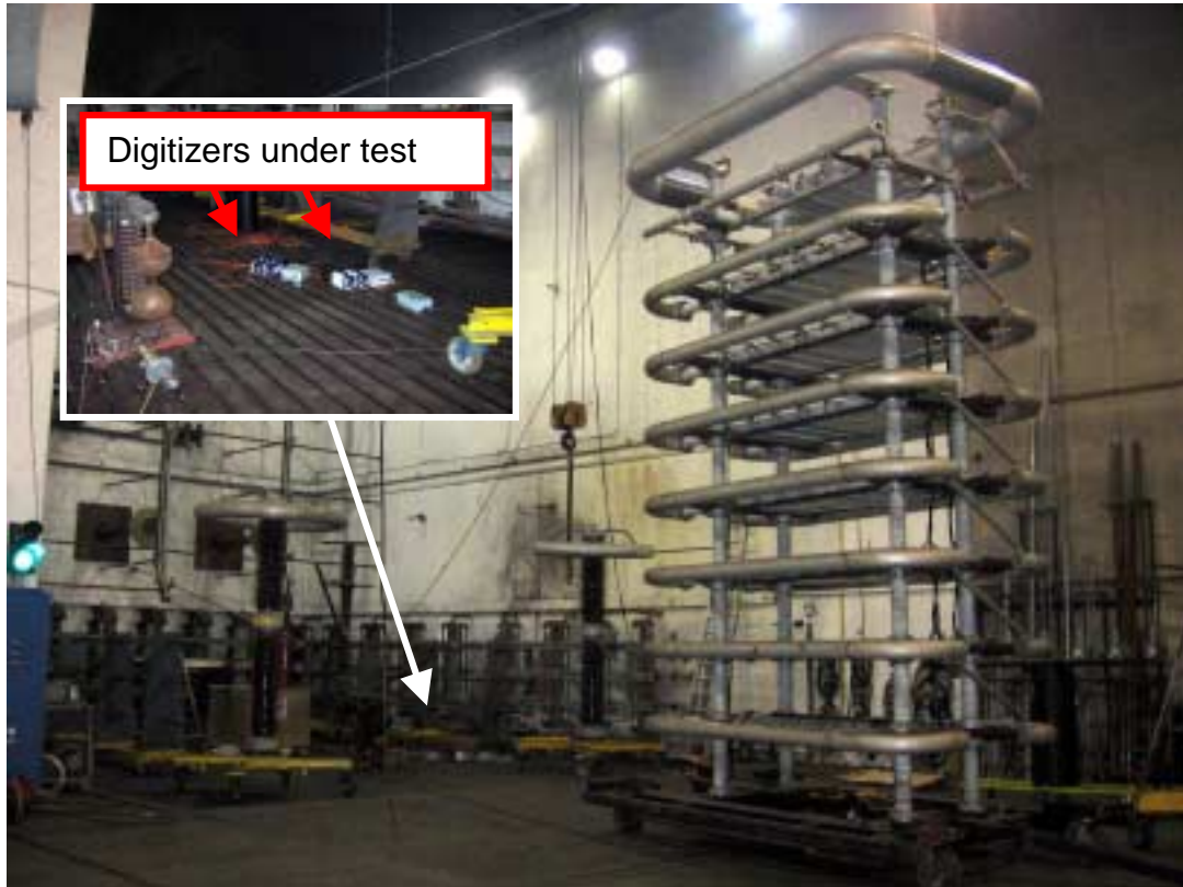
Test set-up for breakdown test
