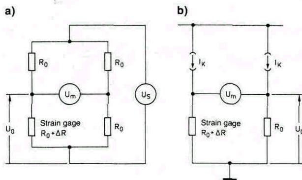
**Fig. 1:** Circuit diagrams for single strain gages
