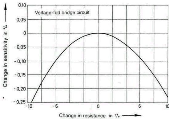
**Fig. 8: Small variation in sensitivity in relation to change in resistance of the strain gage for a voltage-fed bridge circuit**
