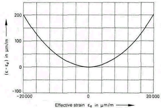
Fig. 3: Deviation of strain  $\epsilon$  from the effective strain  $\epsilon_e$  in relation to the effective strain
