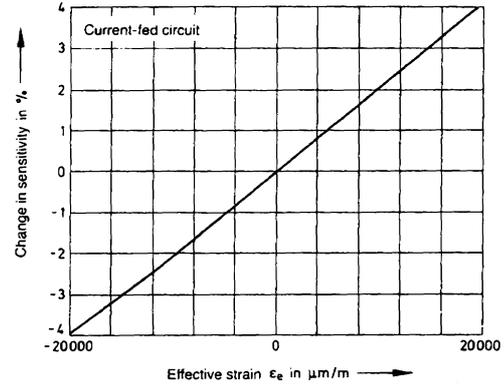
Fig. 7: Large variation in sensitivity in relation to effective strain for the current-fed bridge circuit
