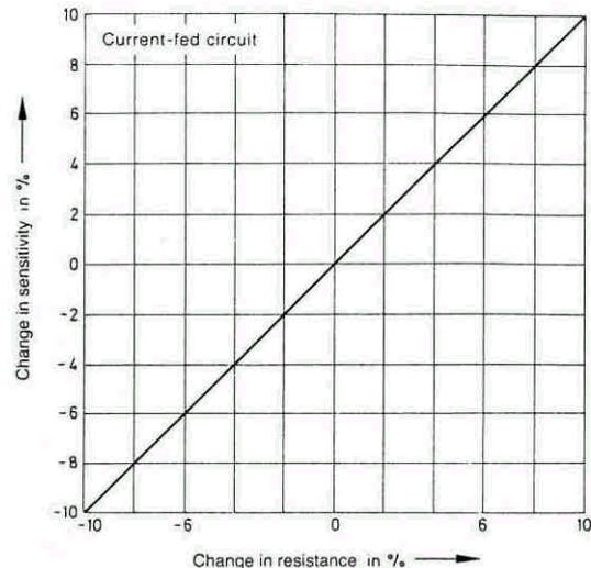
**Fig. 9: Large variation in sensitivity in relation to change in resistance of the strain gage for a current-fed bridge circuit**
