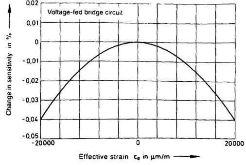
Fig. 6: Small variation in sensitivity in relation to effective strain for the voltage-fed bridge circuit
