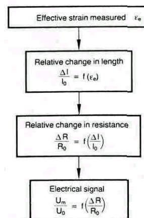
**Fig. 2:** The steps from measurement of the strain to the eventual electrical signal
