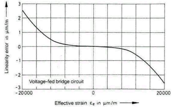
**Fig. 4:** Small linearity error of the voltage-fed bridge circuit in relation to the effective strain
