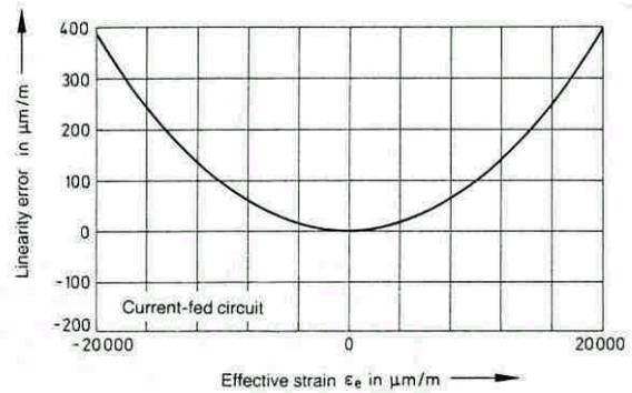
**Fig. 5:** Large linearity error of the current-fed bridge circuit in relation to the effective strain
