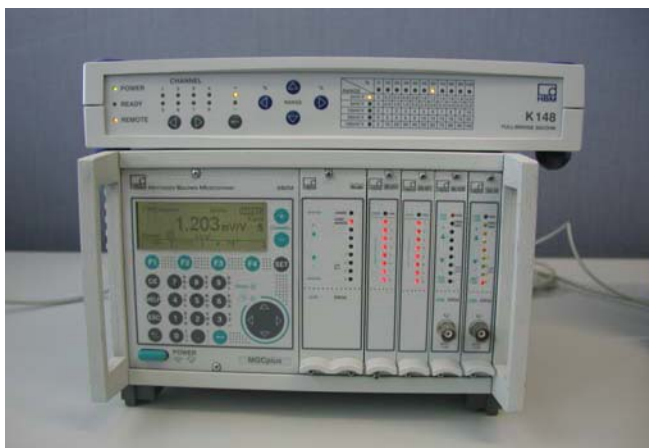
Fig. 3. Setup of the voltage ratio calibration with MGCplus measuring amplifier and computer controlled calibration unit K148
