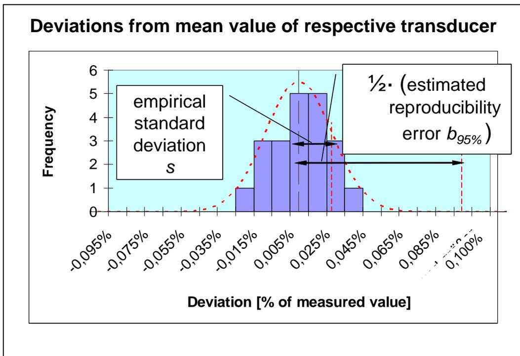
Fig. 1: Transducer type A, measuring range I, calibration step 60% of full range
