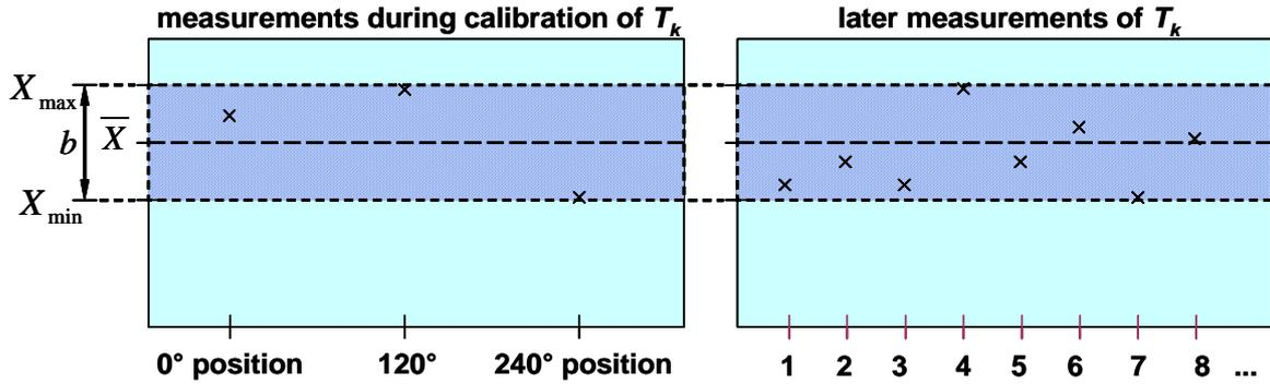
Fig. 3: Effect of reproducibility on uncertainty for transducer calibrated in three mounting positions.
