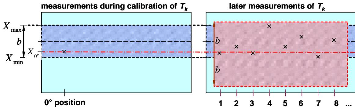
Fig. 4: Effect of reproducibility on uncertainty for transducer calibrated in only one mounting position.
