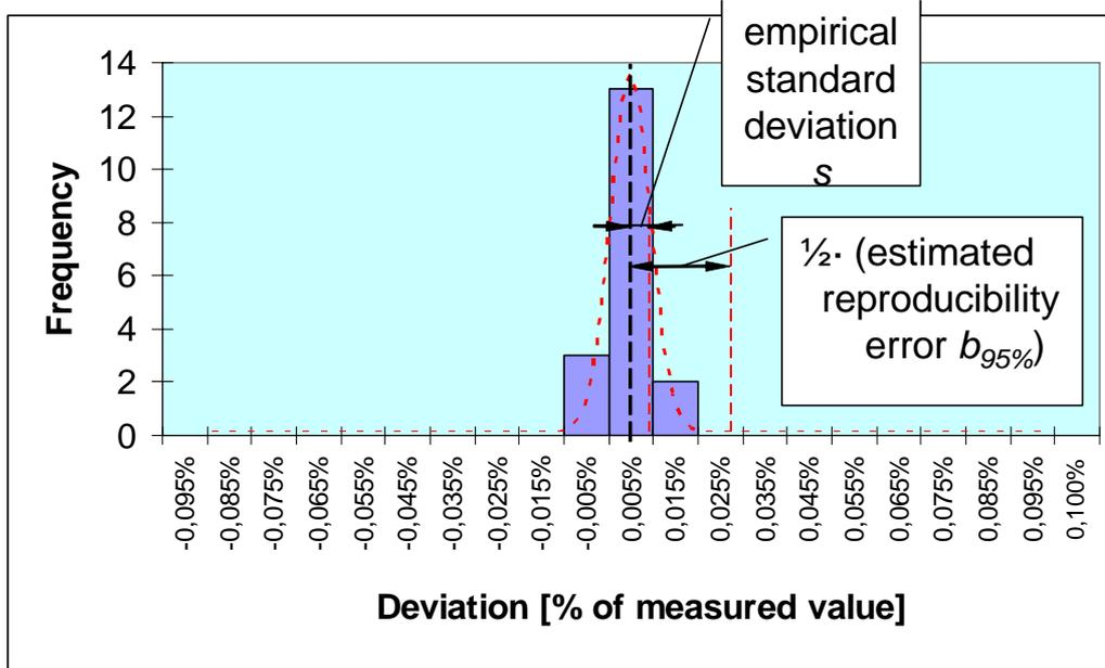
Fig. 2: Transducer type A, measuring range II, calibration step 60% of full range
