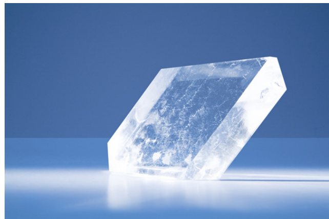
Fig. 2: Gallium phosphate ( \text{GaPO}_4 ) stands out due to its very high, long-term stability
