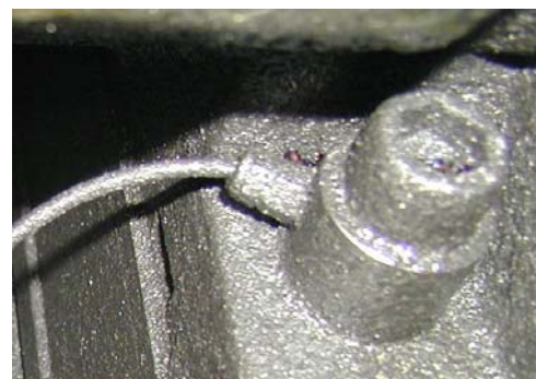
Fig. 6: For tool monitoring, a force washer measures the forces acting on a screwed connection.
