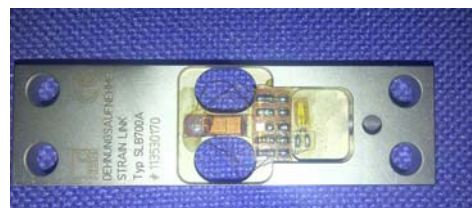
Fig. 3: SLB spring element: The picture clearly shows the area of strain where the strain gauge has been installed
