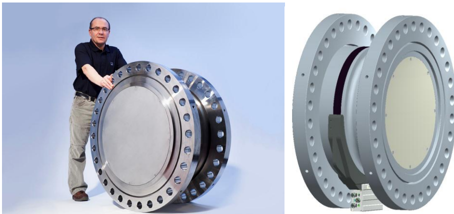
Fig. 5: Implementation of a 1.5 MN transducer and design proposal
