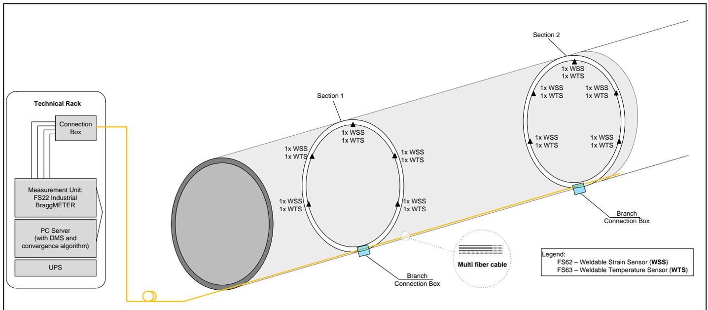
Fig. 1: System Architecture
