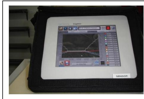
Fig. 11: BraggMETER Portable interrogator
