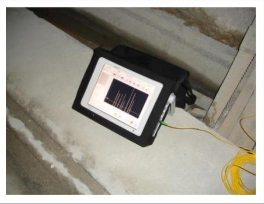
Fig. 30: Optical connection verification
