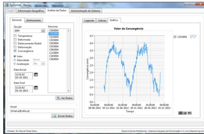
Fig. 41: Regular behaviour of the alignment C01S004
