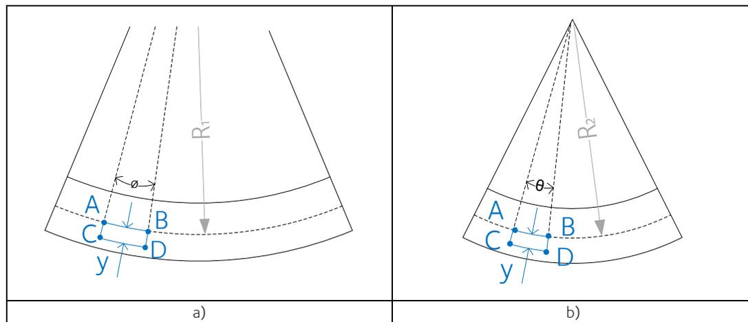
Fig. 7: Bending of initially bended bars: a) before bending; b) after bending
