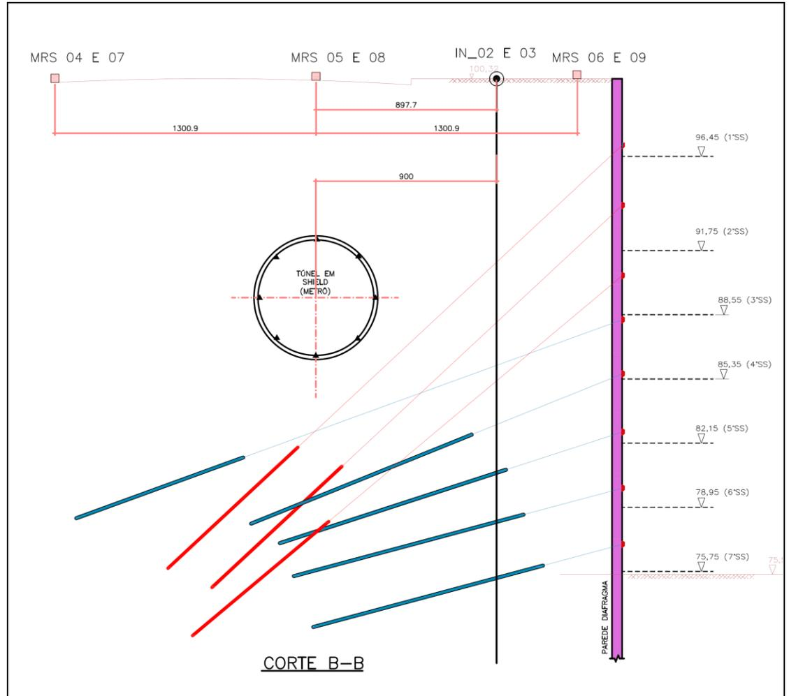
Fig. 44: Excavation and diaphragm wall anchoring plan
