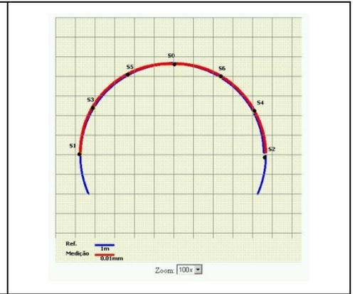
Fig. 24: Example of a search result on the section deformation between two specified dates
