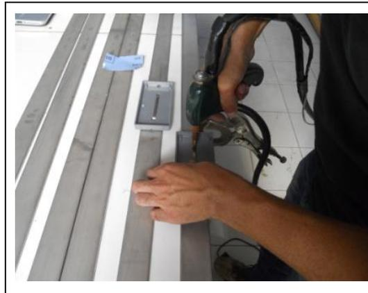
Fig. 49: Welding of sensors
