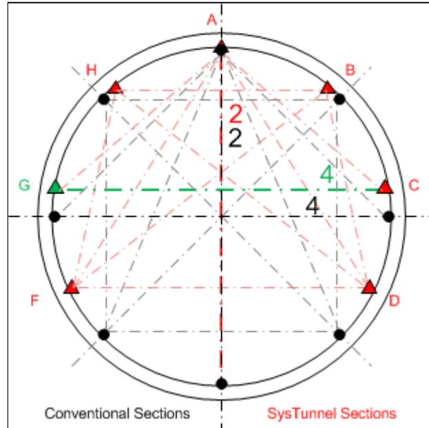
Fig. 57: Sensor positioning on SFO2 (2012)
