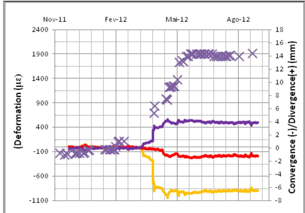
Fig. 58: Evolution of deformation on sensor (C,G) from string 4 and convergence of the "string" 4 of SFO2 and CC6
