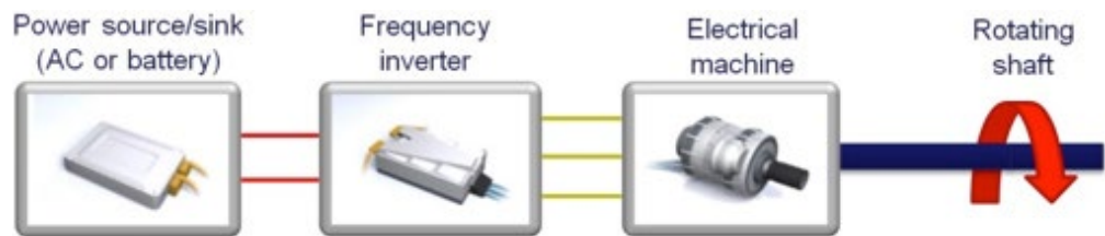
Figure 1. Simplified electrical drive train
