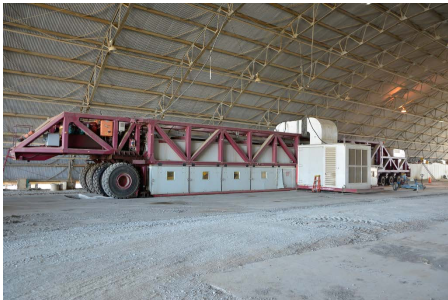
Fig. 1. The Heavy Vehicle Simulator on the ERDC Vicksburg campus can simulate the wheel loads of vehicles ranging from heavy trucks to fully loaded cargo planes, and produce up to 500 passes/hour, around the clock. A combination of insulated removable panels and an air conditioning power plant allow heating the surface under test to up to 130°F or cooling it to 30°F.
