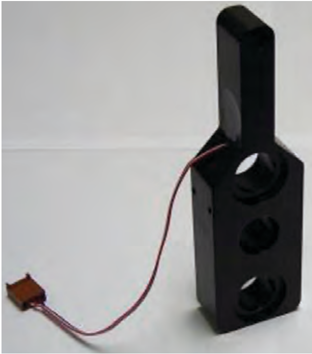
Figure 6. The finished part was made of aluminum with an anodized solution for protection.
