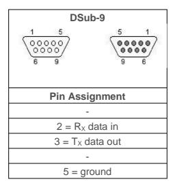
GPS 18 LVC & GPS 18-5Hz PINOUT
