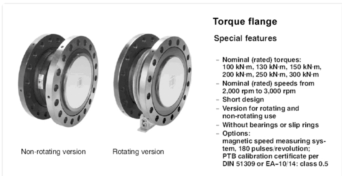
Bild 1: Special features of a torque flange
