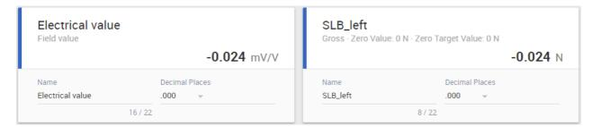
Check that the sensors are unloaded and set the channel to zero.
