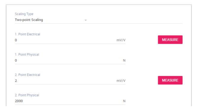
Make sure the sensors are without any load. Then go to the scaling settings for both SLBs. Press measure for the first point electrical.
