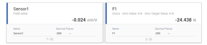
Next step is to scale the sensor according to its sensitivity. Look it up on the sensor itself or in its datasheet.
