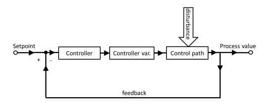
The setpoint provides a value that is compared to the process value, the actual value. The difference between setpoint value and process value results in a control variable that affects the control path. That way disturbance values should be countered to maintain the set point value in a certain range. Besides accuracy, in practice a control loop has also to be adjusted in terms of speed and stability.
