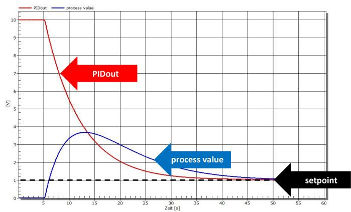
Interference by shortly discharging the capacitor
