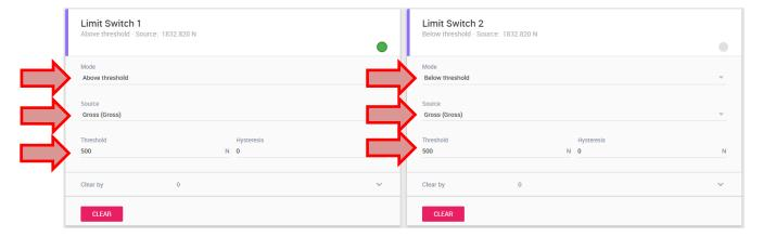
Now the tolerance window is added which should capture the maximal value.
