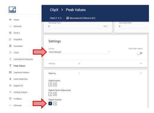
So that the maximum value is not periodically reset (as in the first procedure), the maximum value is held in the "Captured Values" menu.
