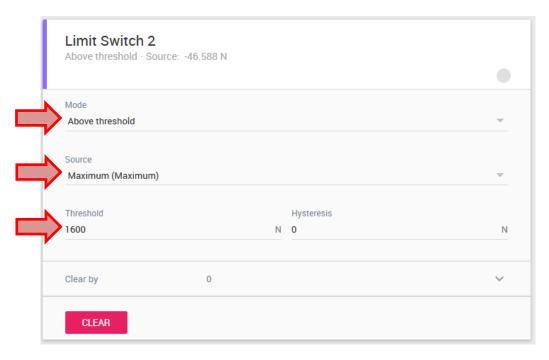
The flag of the limit switch can be transmitted via fieldbus or the digital output.
