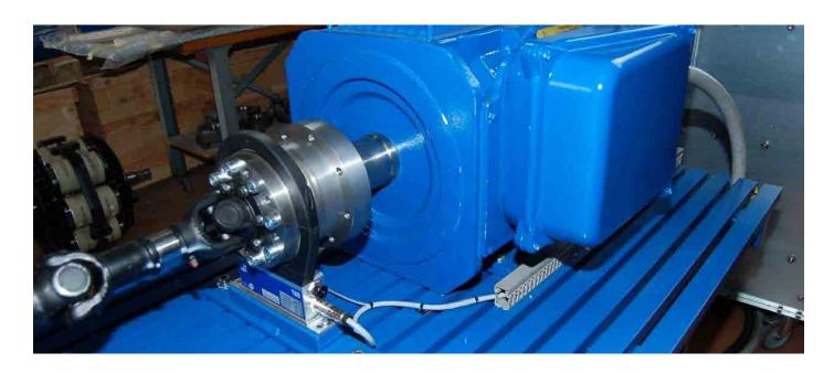
In order to develop a test bench for electric car engines, Dynosens needed an interface to connect its T40B torque transducer to the EtherCAT fieldbus. The TIM-EC that HBM was in the process of launching was put to operational use straightaway ...
