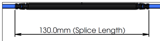
Fig. 6: Splice protection with injected polyimide
