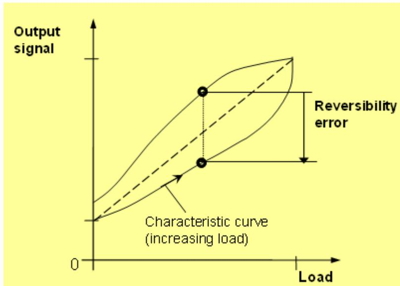
About the relative reversibility error: The difference in measured values with identical force applied between increasing and decreasing force.
