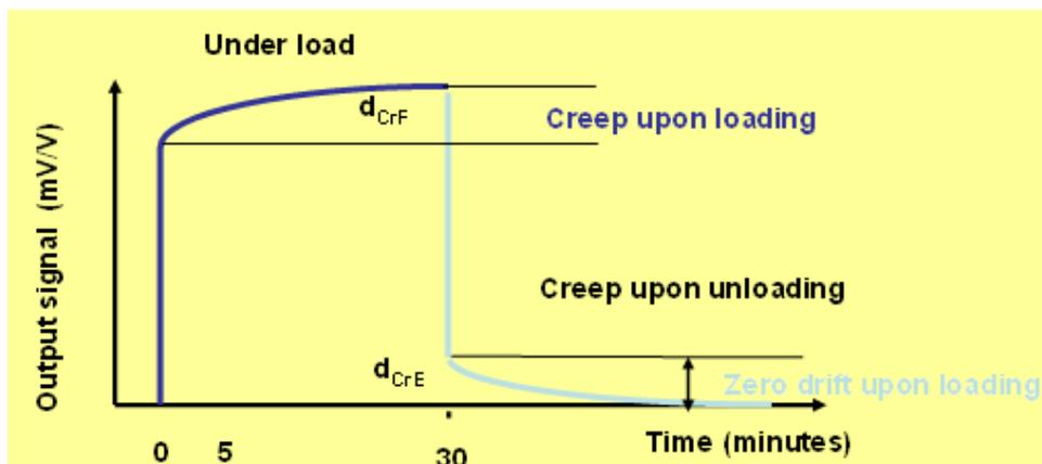
About force transducer creep: the principle.
