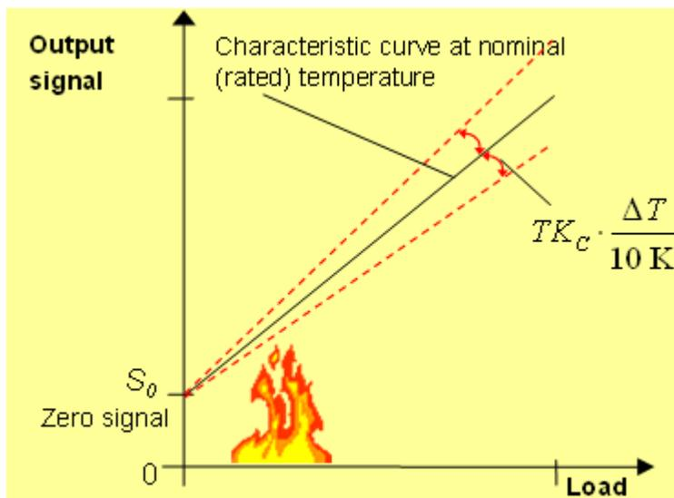
About  $TK_C$ : The gradient of the characteristic curve varies if the temperature changes.
