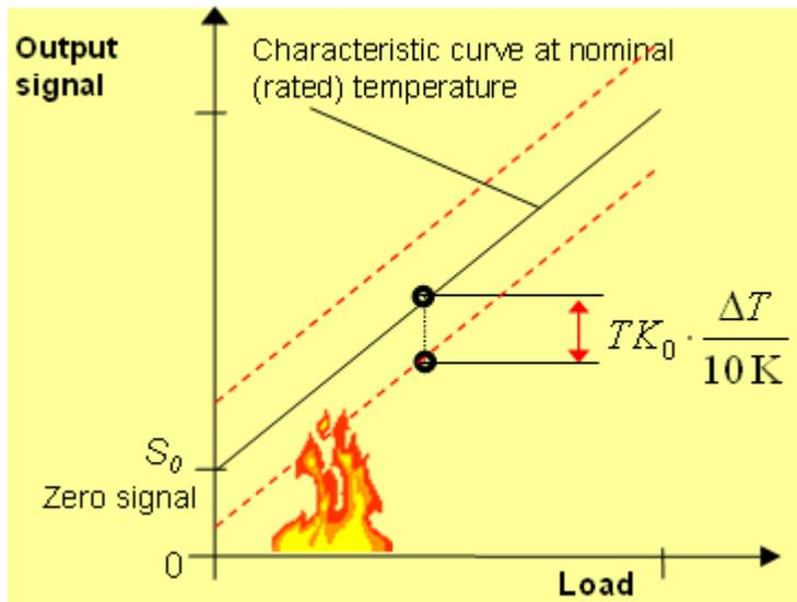
About  $TK_0$ : Parallel shift of a force transducer's characteristic curve in the event of temperature variations.
