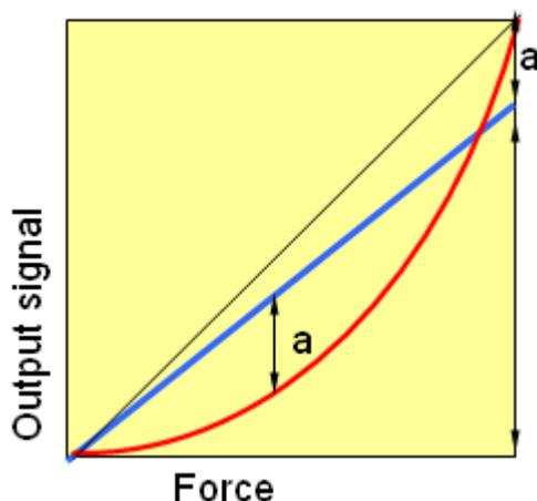
About linearity: The blue line is the ideal straight line, the red line is the actual characteristic curve. "a" is the deviation. "a" is specified relative to the nominal (rated) force in the data sheet.
