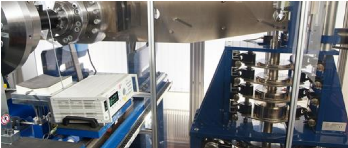
25 kN·m torque reference standard measurement system. One of a total of 4 accredited torque reference standard measurement systems at HBM.
