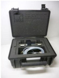
Reference transducer as transfer standard in NMIs
