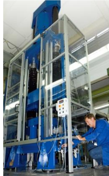
Build-up system for force calibration Class 00 acc. ISO 376
