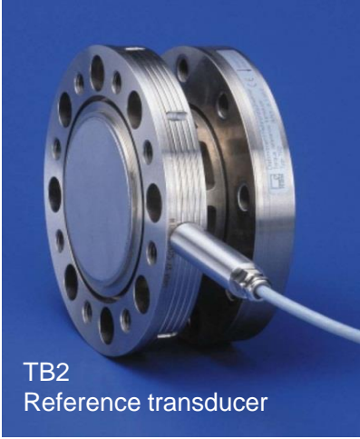
Reference transducer as transfer standard in NMIs
