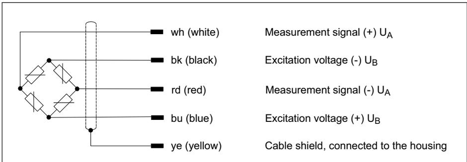
Fig. 7.1 Transducer with a four-core connection cable
