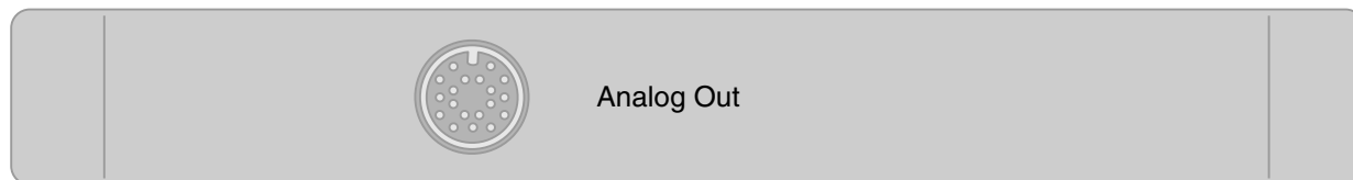
Figure 5-5: Diagram showing the analog out connector on the back panel of an EBRG layer.
