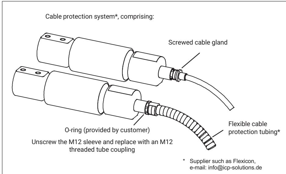
Even without a cable protection system, standard load cells can achieve IP68/IP69K degree of protection. In applications where the PUR cable of the load cell can be chemically or mechanically attacked or destroyed, extra cable protection can be provided by means of standard cable protection systems.
