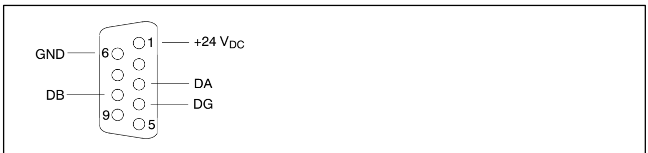
Fig. 6.1: CC-Link interface connector pin assignment, 9-pin D-Sub socket (pin version), contact view
