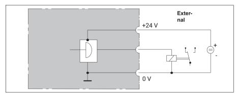
The voltage at the output is approx. 0.5...1 V lower than the externally connected supply voltage. The maximum current depends on the strength of the external supply voltage, but must not exceed 0.5 A.
