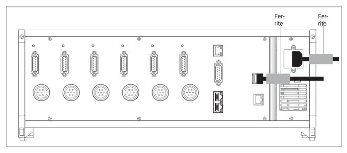
Fig. 1.1 Position of the ferrites
