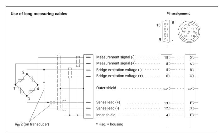
When using long cables and with a high transducer resistance, HBK additionally recommends soldering resistors in the sense leads. The resistors should be placed as close as possible to the transducer. The value of the resistances must be half that of the bridge resistance ( $R_B/2$ ).
