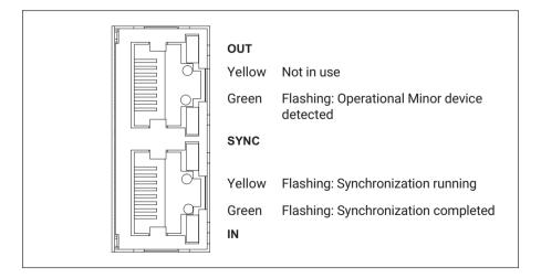
To synchronize several DMP41s, you need a synchronization cable with HBK ordering number1-KAB287-3. Synchronization means that all the supply voltages are phase-identical and phase-locked in all the DMP41s. The status of the synchronization connection is displayed.
