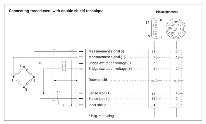
With very small measuring ranges, in environments with major interference and when using long cables, HBK recommends double-shielded measuring cables. The inner shield should be open on the transducer side.
