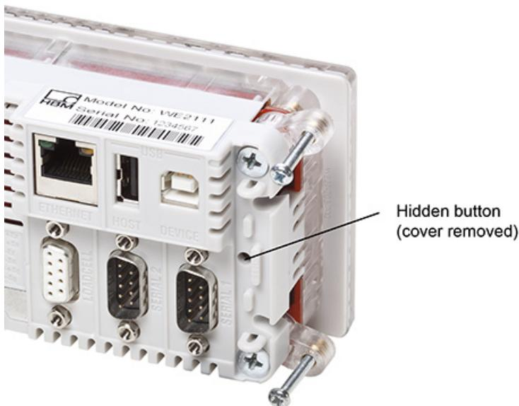
Fig. 11: Rear view with fastening clamps unfolded
