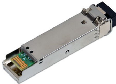
Figure B.45: 1 Gbit Optical Network SFP module 1310 nm
