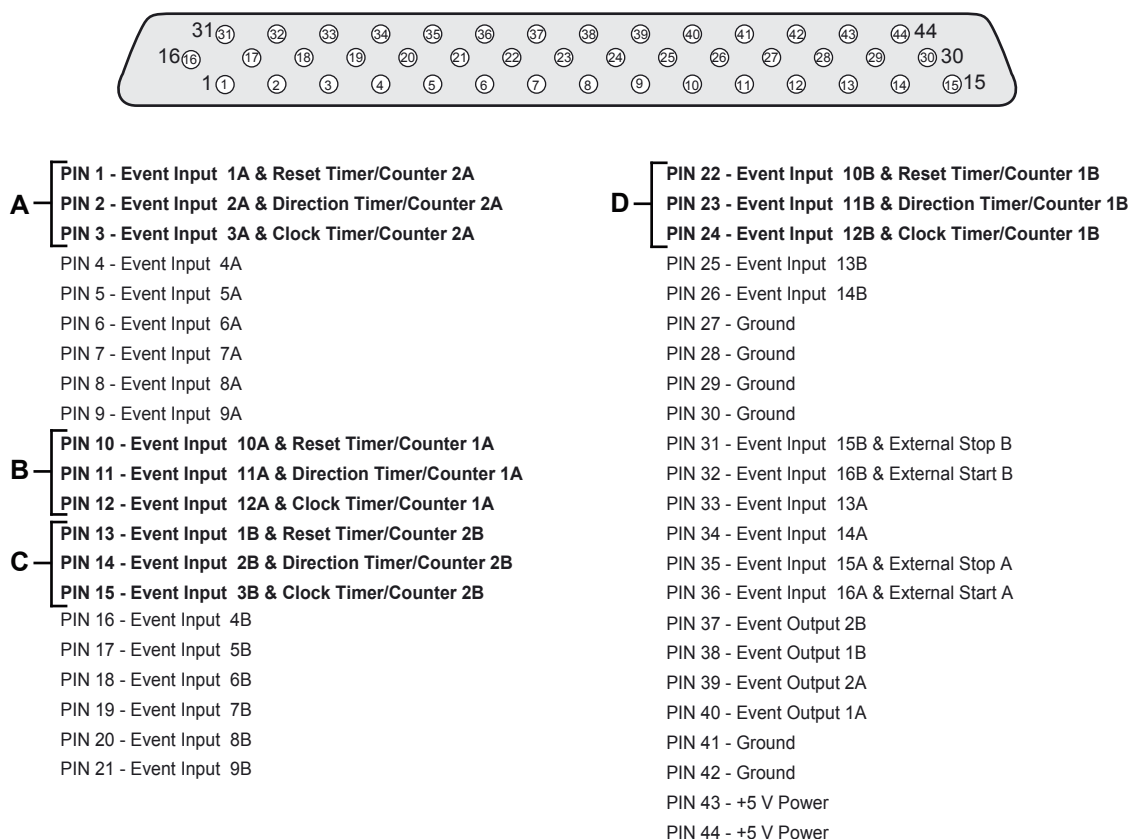
Figure J.20: Pin diagram for Digital Event/Timer/Counter connector
