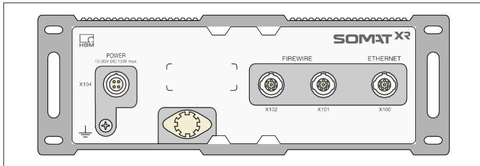
Each MX module has a similar back panel with a power connector, two FireWire connectors, and one Ethernet connector.
