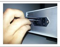
Fig. 4.12 Removing the fuse
