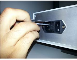
Fig. 4.12 Removing the fuse
