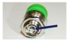
Fig. 4.9 Broken connectors
